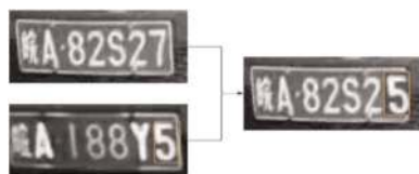
FIGURE 10 Synthetic license plate generation [Color figure can be viewed at wileyonlinelibrary.com ]
