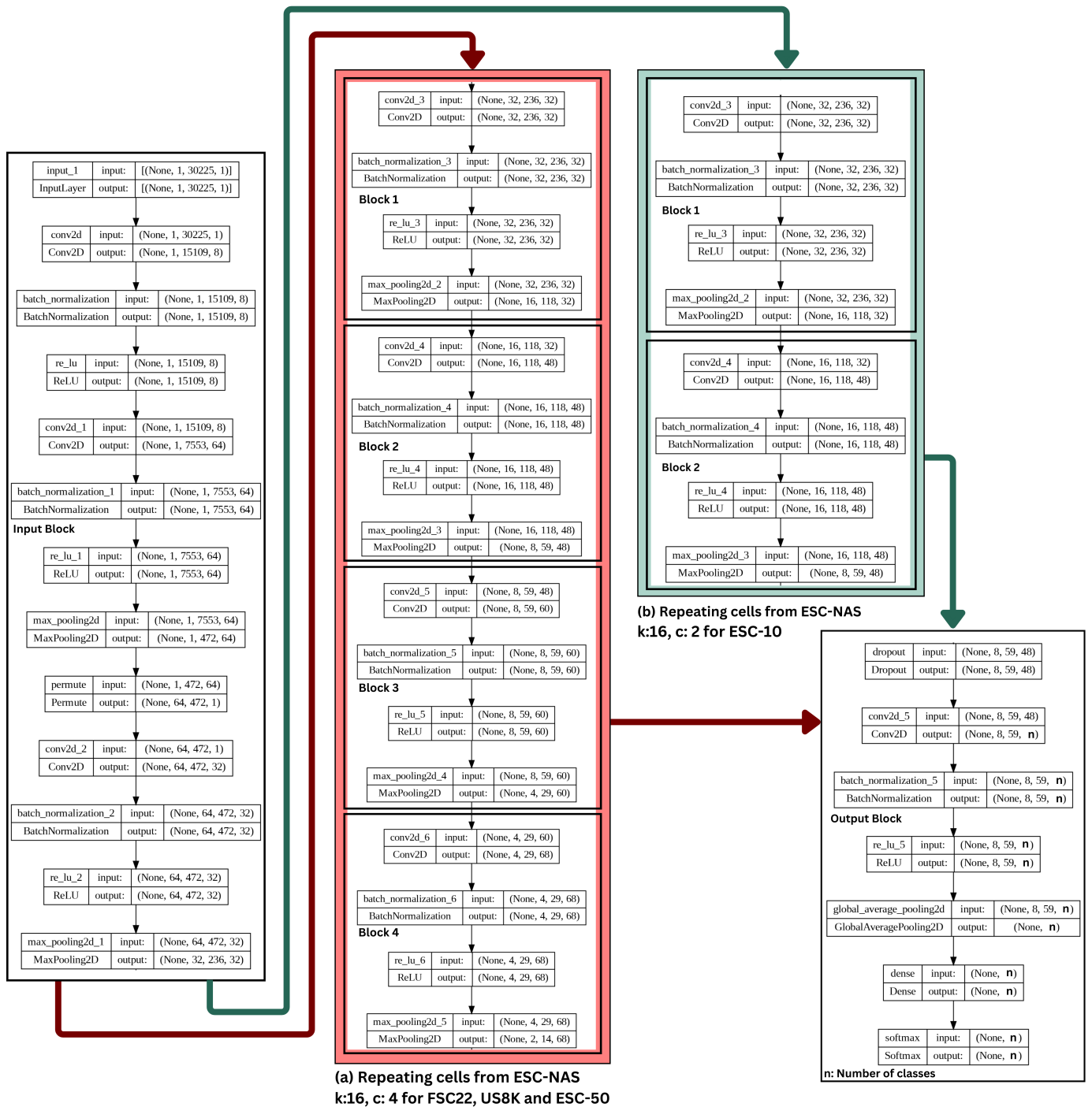
Figure 4. Resulting architectures from ESC-NAS for different datasets. (a) k: 16, c: 4 for FSC22, US8K, and ESC-50 (b) k: 16, c: 2 for ESC-10.
