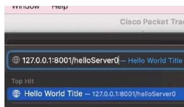
Figure 1.22: Accessing the route /HelloServer0 on port 8001.
