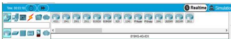
Figure 1.3: Top row = broad categories (Network Devices, End Devices, Connections), bottom row = subcategories (Routers, Switches, etc.).
