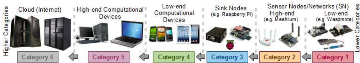
Figure 3: Categorization of IoT devices based on their computational capabilities.
