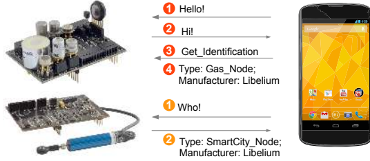
Fig. 1: Heterogeneity in term of communication and message/command passing sequences. Some sensors may need only a few message/command passes and others may require more. The messages/commands understood by each sensors may also vary.
