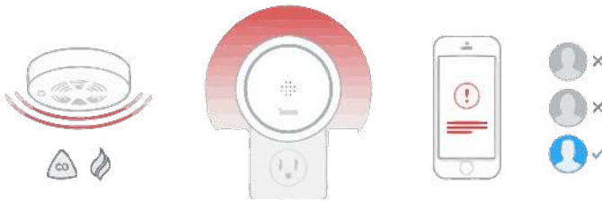
Fig. 16. Enriching smartness to legacy devices: Legacy devices may monitor fire and smoke. Once these legacy devices detect any abnormalities, they will trigger their alarms and start to make sounds. Leo is designed to listen to such alarm sound. Once Leo detects such sound, it triggers its reaction mechanisms such as sending notification to the users, neighbours, and government authorities such as fire brigade in a predefined order.
