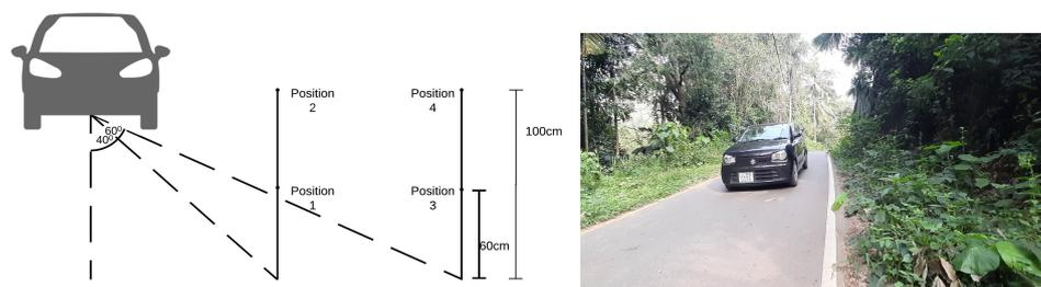
**Figure 11.** Camera positions (left) and sample deployed image (right). 757
