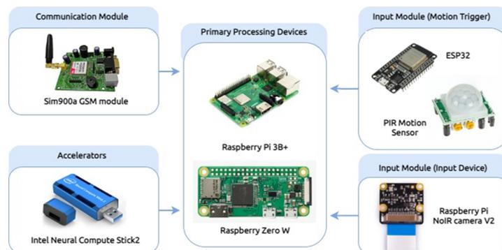
**Figure 2.** Hardware stack of the proposed solution
