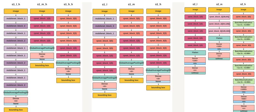
**Figure 9.** Model Architectures (left): hardware optimized detection, (middle): hardware agnostic detection, (right): recognition subnetworks.
