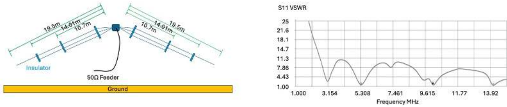
(a) Inverted “V” dipole antenna, designed for multi-frequency operation at 3.607MHz, 5.350MHz, and 7.070MHz.
