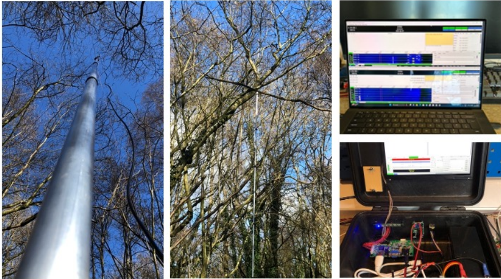
Fig. 7. Remote node test setup housed in a ruggedised Peli 1400 case, featuring a transceiver, Raspberry Pi, GPS module, real-time clock, and 12V lead-acid battery. This configuration ensures durability and reliable operation in forested environments.
