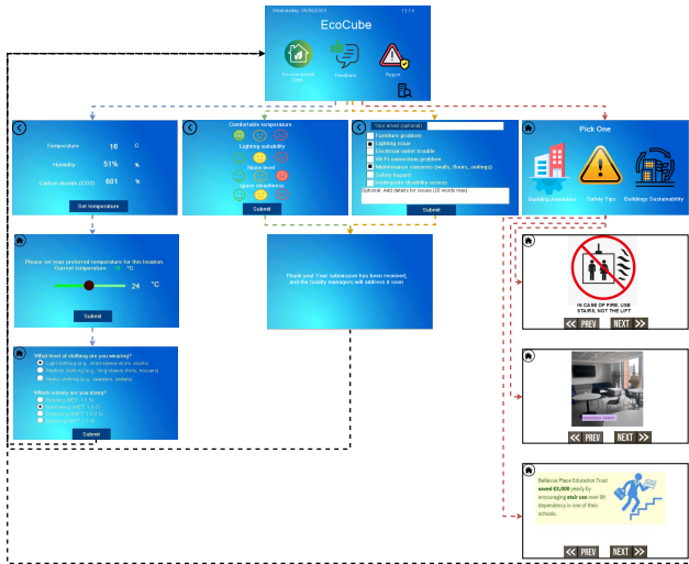
Figure 7: Illustrates the occupant interaction flow when using the EcoCube device.
