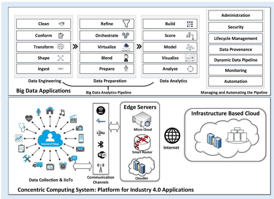
**Fig. 3.** Multistage execution, automating, and management of BDA processes (i.e., data engineering, data preparation and data analytics) in concentric computing environments (such as sensors and wearable devices as endpoints, IoT devices, edge servers, and cloud computing servers) [32].
